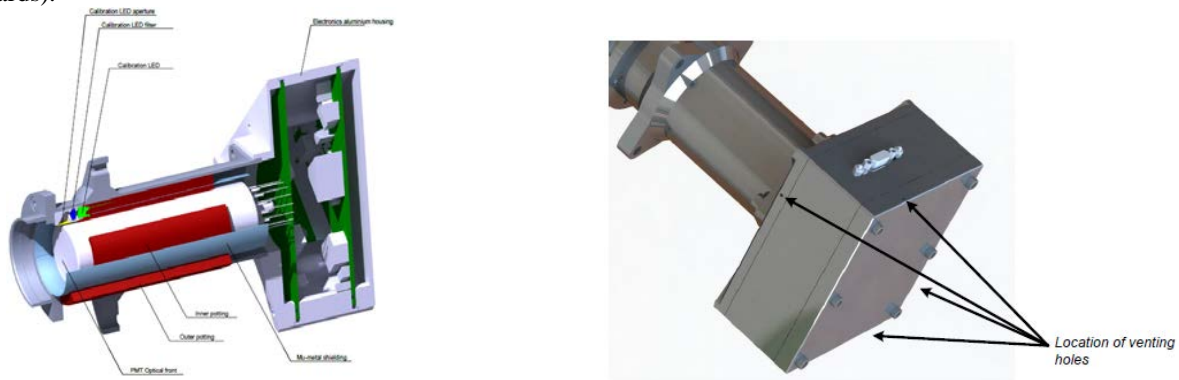
Figure 9 Venting design for PHOT and PCBs showing venting of potting material through the electronics box or outwards through the front of the optics.
