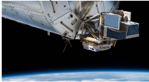
Figure 4 ASIM payload external attached to the ISS Columbus CEPA platform
