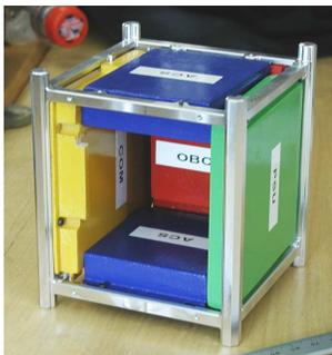
Fig. 6. Early prototype of AAU Cubesat.
